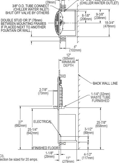
Note: New Installations Must Use Ground Fault Circuit Interrupter (GFCI). It is highly recommended that the circuit be dedicated and the load protection be sized for 20 amps.
